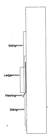
Rubber flashing lies inside of siding over ledger, then runs between ledger and house, then runs between ledger and siding below ledger
