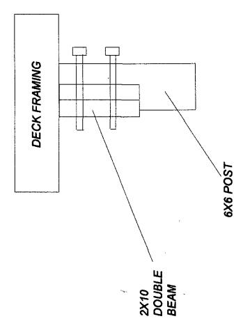
2X10 UNDERCARRIAGE BEAM NOTCHED AND BOLTED ONTO 6X6 POST WITH HALF INCH GALVANIZED BOLTS
